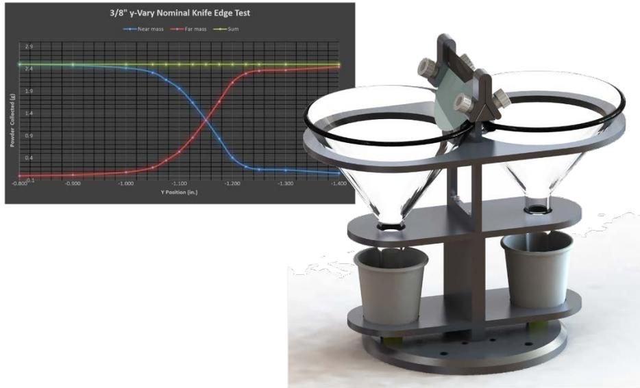
Figure 4: 1D Knife-Edge Profiler with representative dataset
