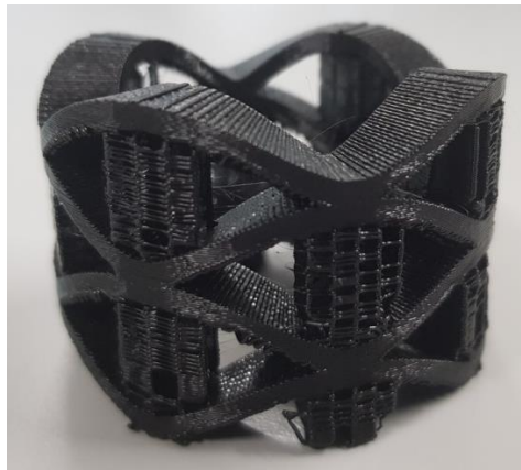
Figure 9 - A 3-axis wave spring sample, including supporting structures
