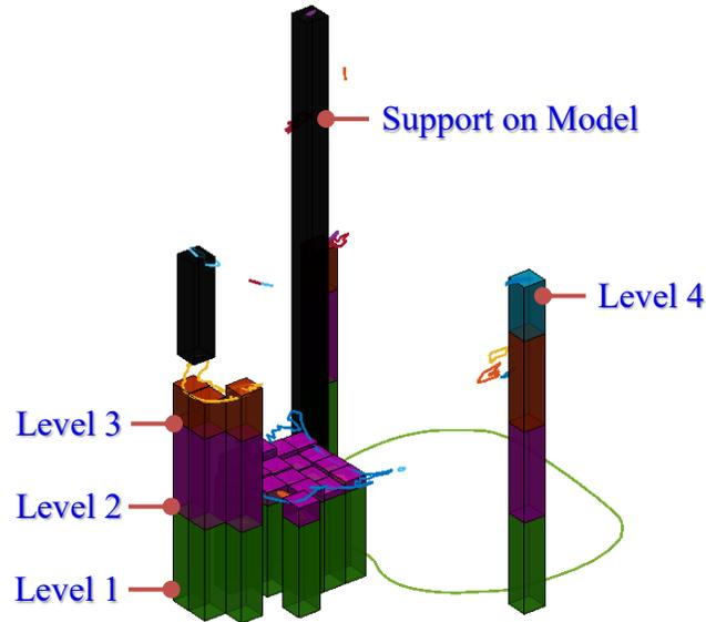
**Figure 3.** Conventional support structures split into levels with the given modular block height for the Atatürk model. The boundaries show the areas which require support.
