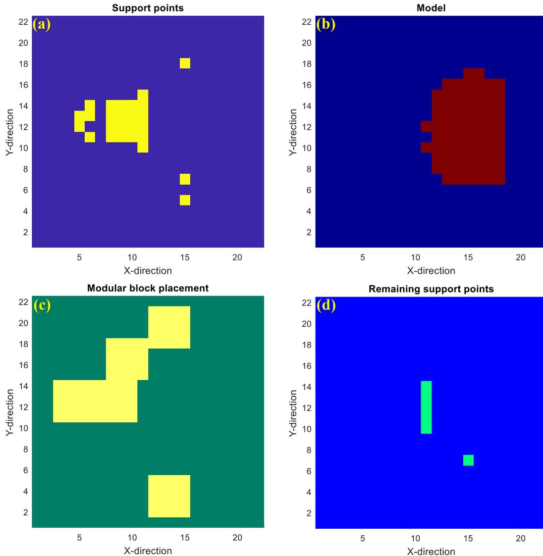
**Figure 5.** Block placement with consideration of collision with the CAD model: (a) Conventional support structure map (b) CAD model map (c) Modular block placement map (d) Remaining support points map.
