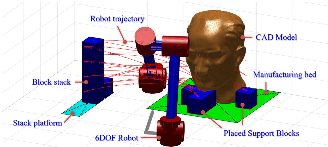
**Figure 7.** Robotic additive manufacturing setup with modular support block placement
