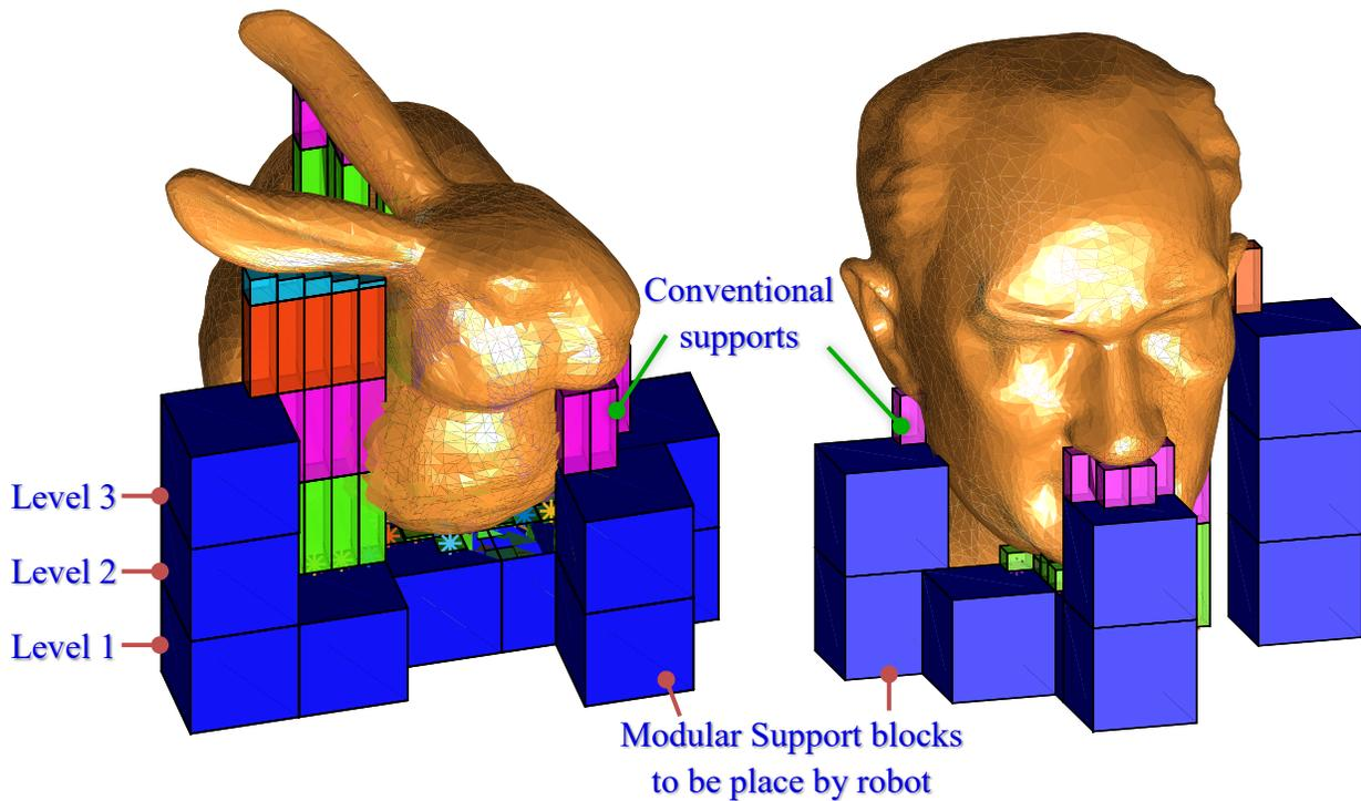
**Figure 6.** Modular support structures results: (a) The Stanford bunny (b) The Atatürk portrait
