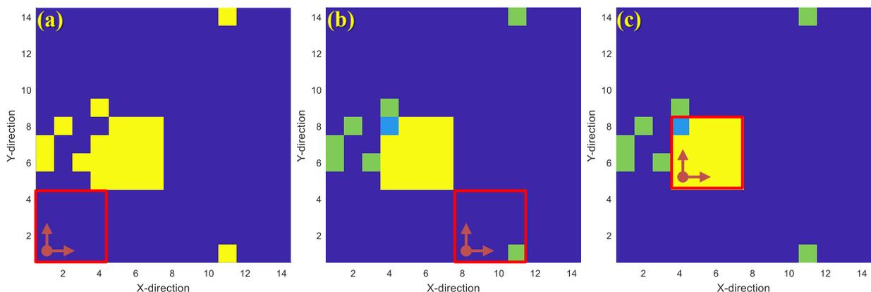
**Figure 4.** Sliding window search for placement of the modular block: (a) Windows is at the origin (b) Window has moved in the x direction (c) Window has found the maximum location
