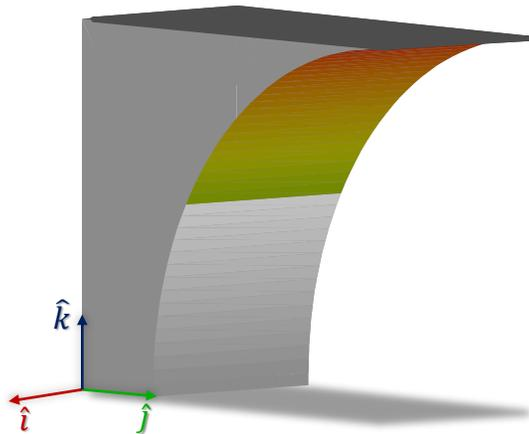
**Figure 1.** Overhanging faces that require support colored from green to red. Grey faces do not require support.
