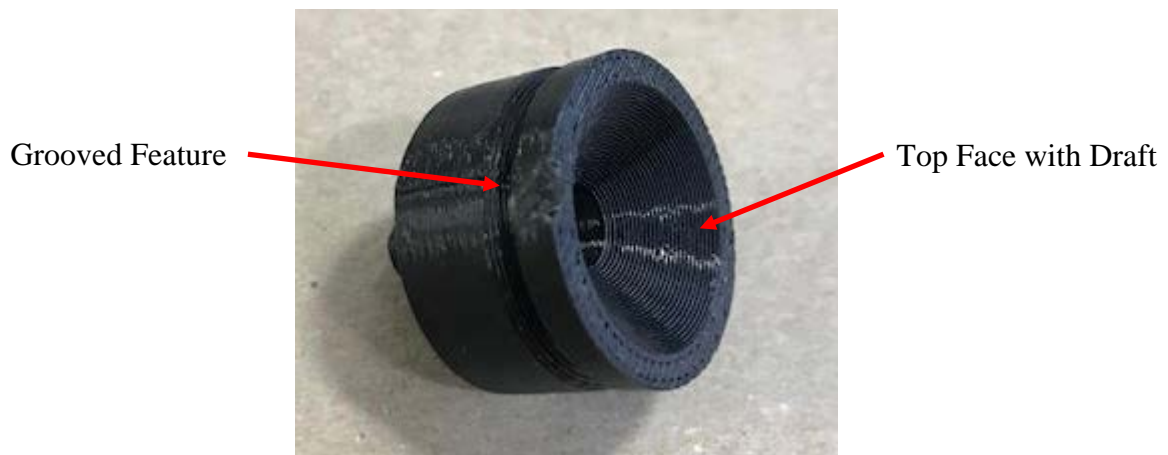
Figure 3: Fiducial design features that ensure proper alignment.
