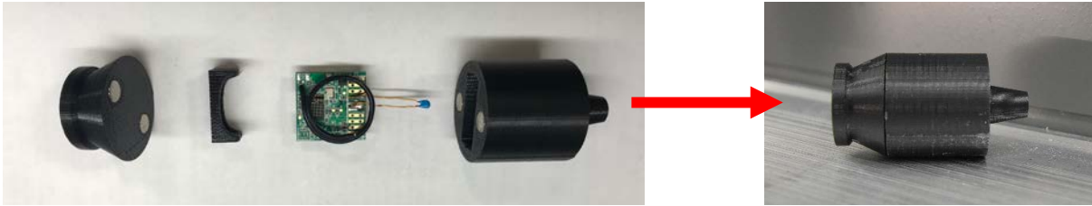
Figure 9: On the left is the sensor module assembly, displaying the magnetic lid, cap, sensor, and main body respectively. On the right is the sensor module fully assembled.
