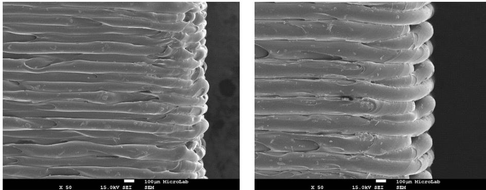
Figure 1 – SEM micrographs of 0.1 (left) and 0.2 (right) mm layer deposition using FDM.
