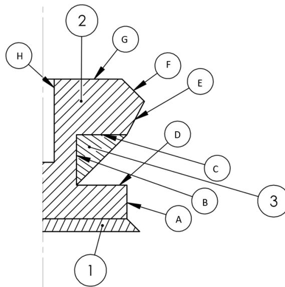
Figure 6 – Half-section of the example part with surfaces that need to be finished.
