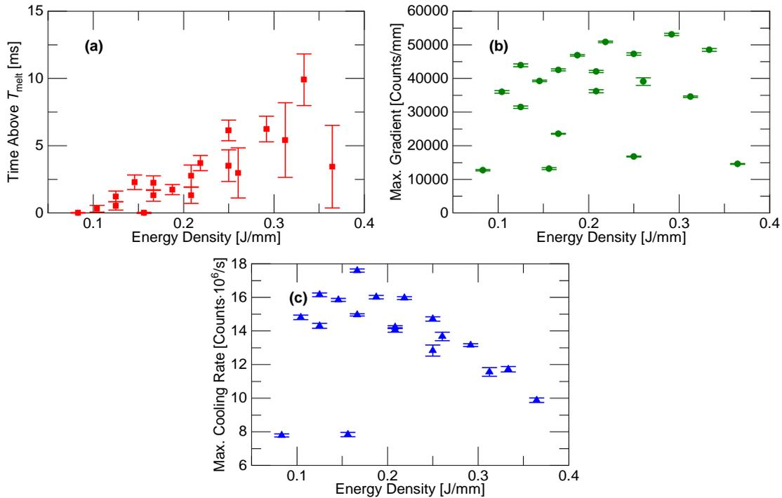
FIG 8: (a) Time above melting temperature, (b) maximum gradient, and (c) maximum cooling rate as a function of linear energy density.
