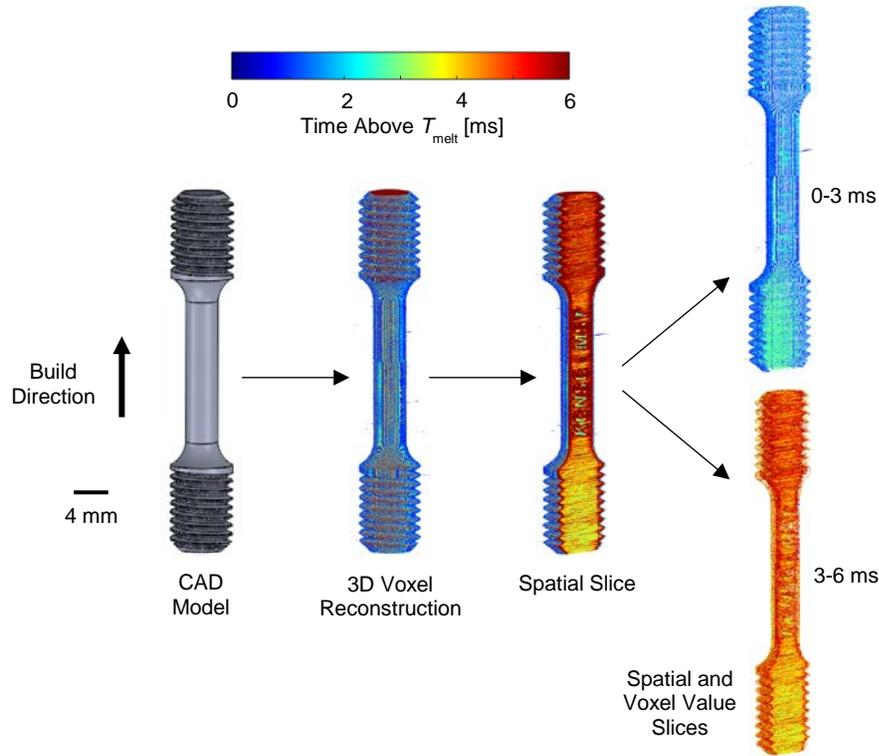
FIG 5: 3D voxel reconstruction of tensile test specimen showing introduced defect in gage length through spatial and color scale slicing.
