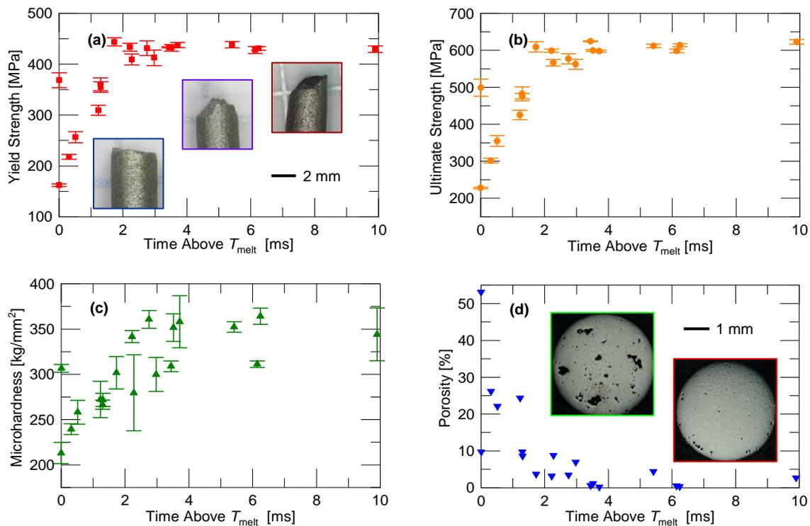
FIG 9: Specimen properties as a function of time above melting temperature.
