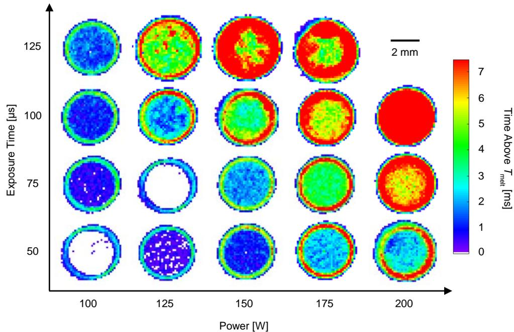
FIG 7: Representative color maps of time above melting temperature for layers in tensile test specimens' gage lengths processed with varied laser power and exposure time.
