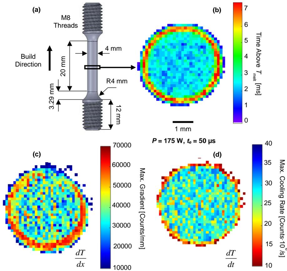
FIG 4: (a) Tensile test specimen geometry and color maps of layer in gage length for thermal features of (b) time above melt temperature, (c) maximum gradient, and (d) maximum cooling rate.
