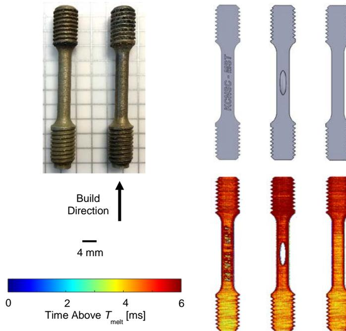
FIG 6: Identification of changes in thermal history and internal defects in tensile test specimens through layer-to-layer process monitoring.
