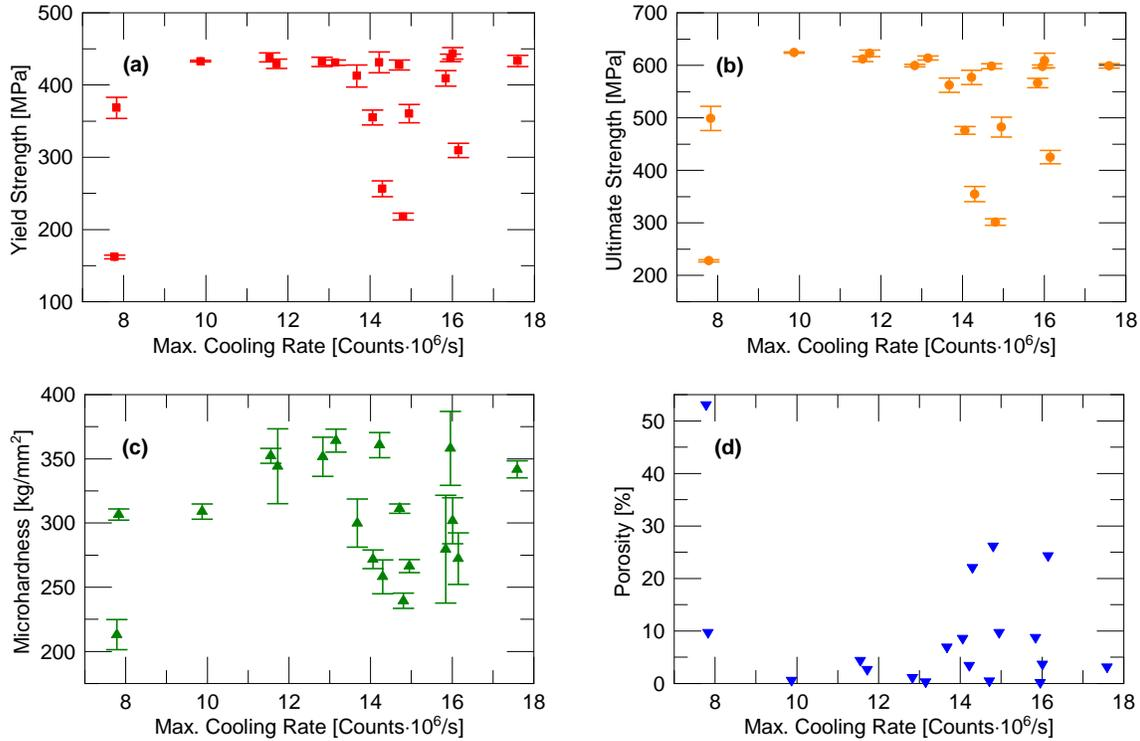
FIG 11: Specimen properties as a function of maximum cooling rate.
