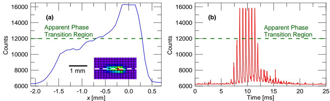
FIG 3: (a) Apparent phase transition region in spatial profile of melt pool and (b) temporal thermal data for single pixel.
