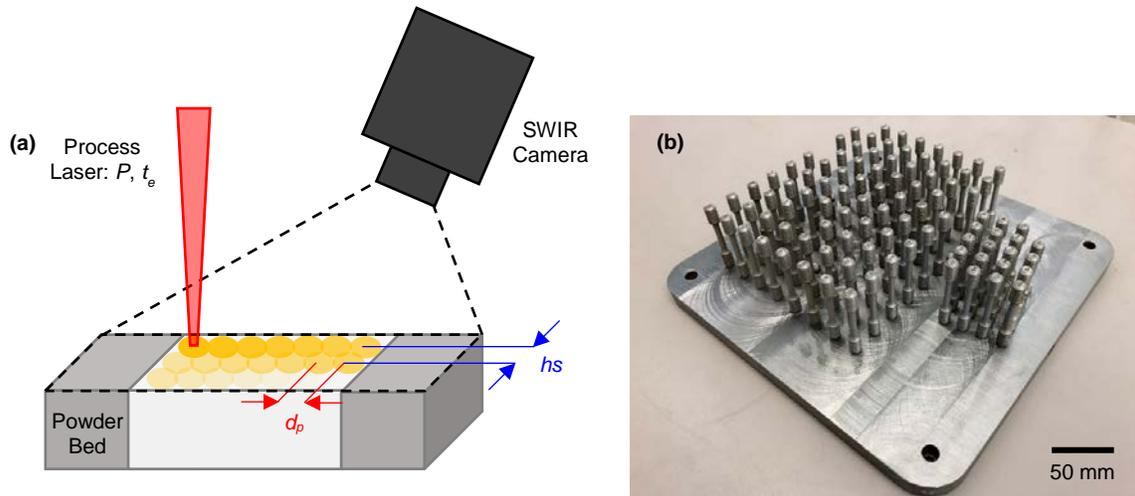
FIG 1: (a) Schematic of AM250 building process with SWIR camera observing powder bed and (b) completed build of tensile test specimens.
