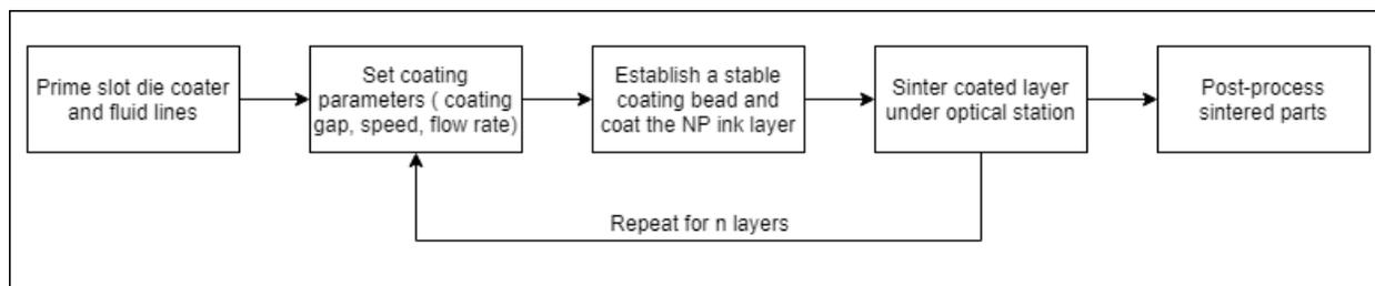
Figure 1: Simplified process flow schematic of the  $\mu$ -SLS system.
