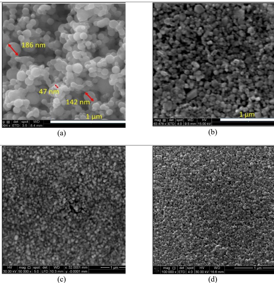
Figure 5. Scanning electron micrographs for: a) Cu nanopowders, b) Spin coated Cu NP ink sample, c) Slot die coated Cu NP ink, d) Slot die coated Ag NP ink.
