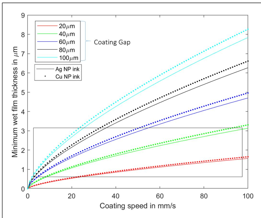
Figure 3: Minimum wet film thickness (in  $\mu\text{m}$ ) versus coating speed (in  $\text{mm/s}$ ).
