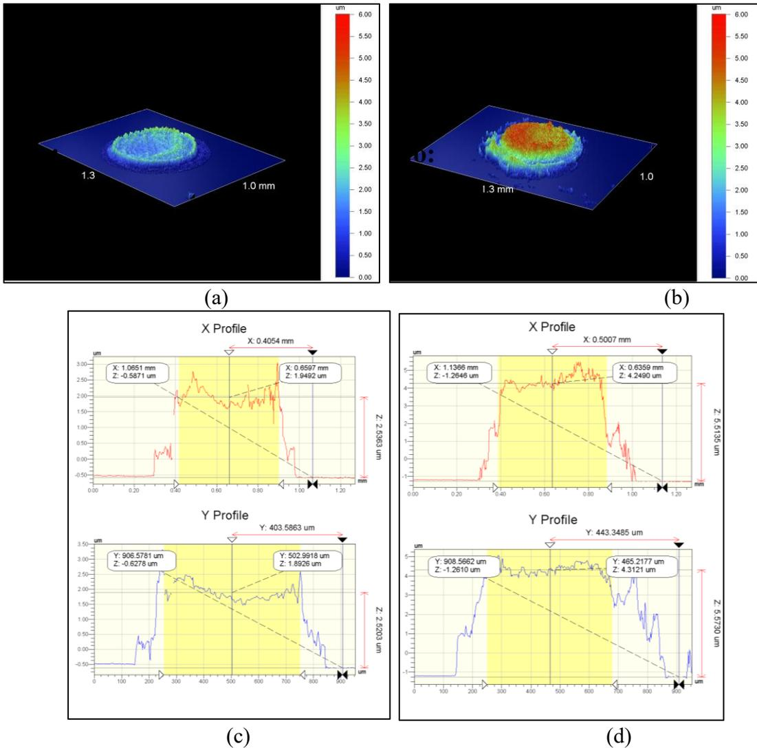
Figure 6. 3D profile of a) single layer sintered sample, b) bilayer sintered sample.
