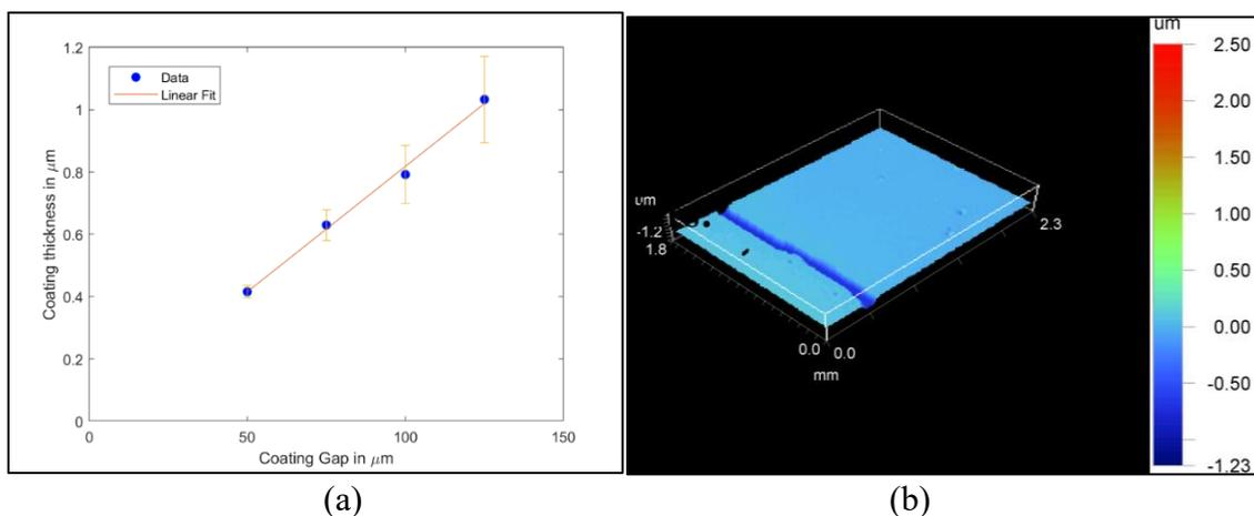
Figure 4. a) Experimental dry film thickness (in  $\mu\text{m}$ ) versus coating gap (in  $\mu\text{m}$ ) b) Optical profilometry 3D plot showing the coating uniformity
