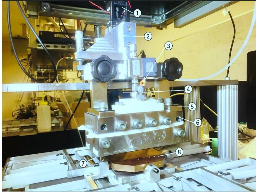
Figure 2: Components in the assembly of the slot die coating system- 1. z-direction motor coupled with 100mm travel leadscrew 2. Pivoting bracket 3. Input for air pilot valve 4. Slot die input 5. Die support Arms 6. Die head 7. Die lips 8. Substrate
