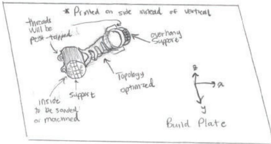
**Fig. 6.** A sketch of how the bicycle stem would be positioned within a L-PBF chamber for fabrication. Some notes are provided by students in the sketch.
