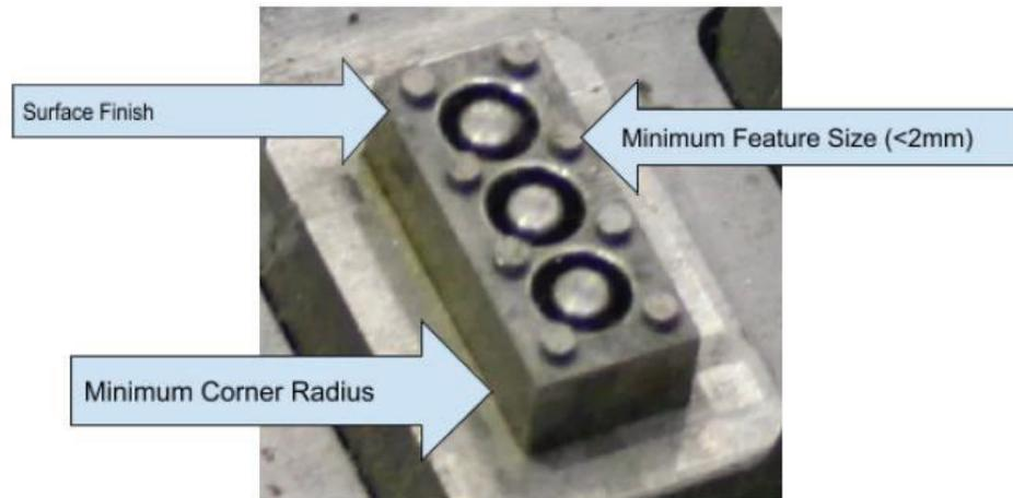
**Fig. 4.** A photo of a LEGO die with challenges for AM pointed out.
