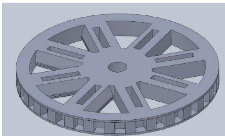
**Fig. 9.** Proposed re-design of an aerospace rotor for AM.
