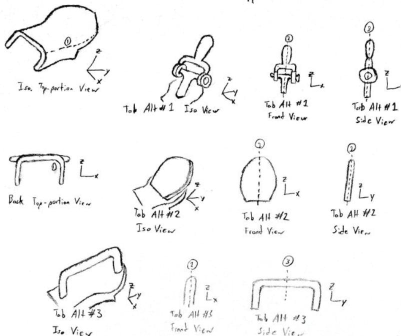
**Fig. 3.** Conceptual design sketches for re-design of a zipper for metals AM.
