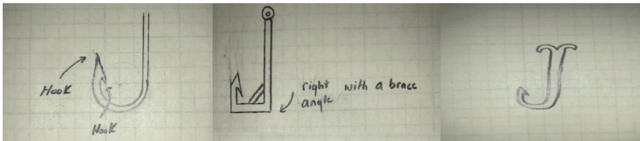
**Fig. 7.** Student sketches demonstrating (left) a typical fish hook, (middle) an AM fish hook with support brace concept, (right) a hole-less fish hook concept for AM.
