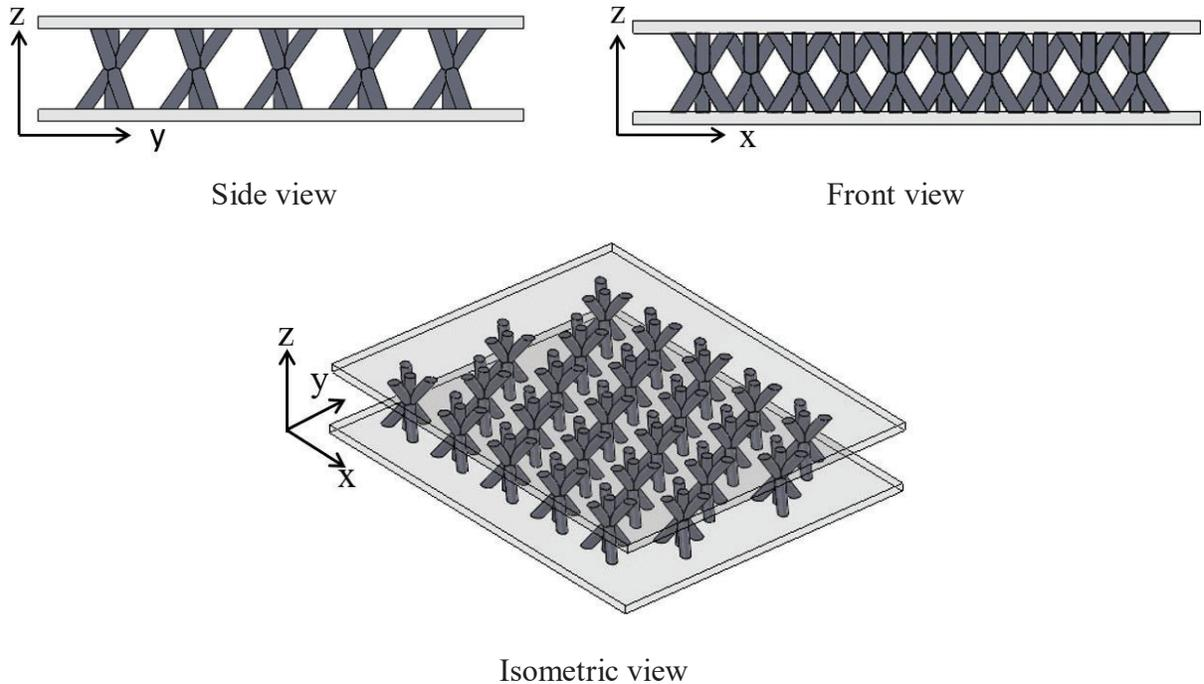
Figure 2: Side, front and isometric views of the sandwich structure with SRK core
