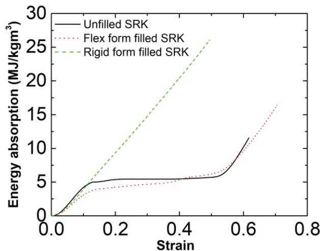
Figure 6: The energy absorption per unit weight of unfilled SRK and foam filled SRK against the strain.
