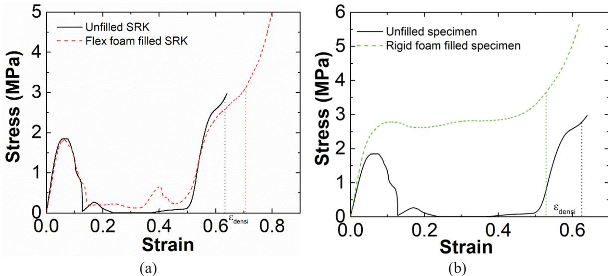
Figure 4: The compressive response of unfilled SRK and (a) flex foam filled SRK and (b) rigid foam filled SRK
