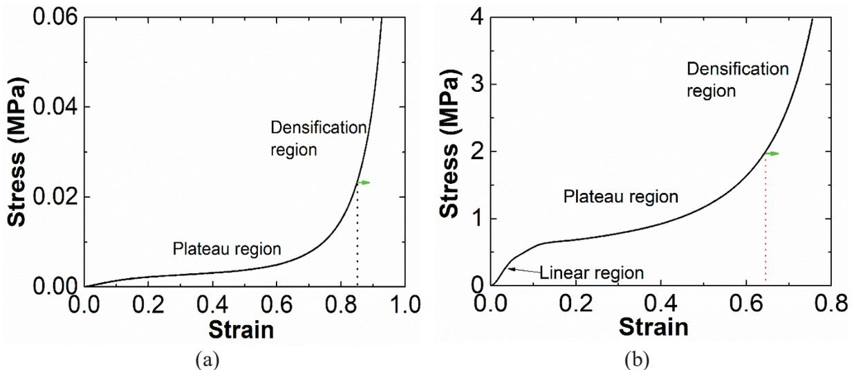
Figure 3: The compressive strain-strain curve for (a) flexible foam and (b) rigid foam
