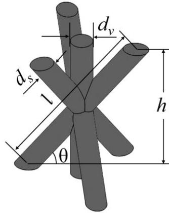
Figure 1: Unit SRK structure with its geometric parameters
