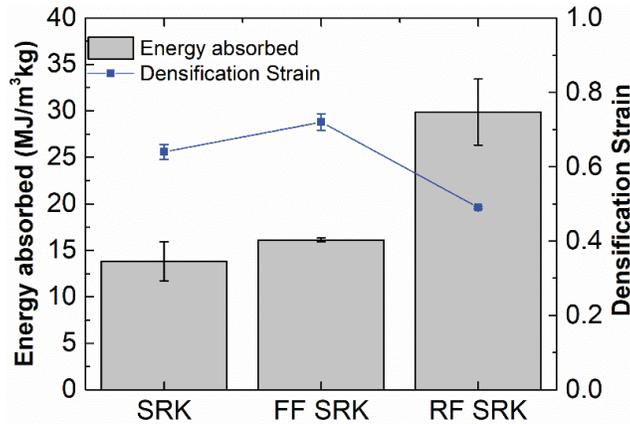
Figure 5: Total energy absorption to densification and densification strain of unfilled SRK, flex foam filled SRK and rigid foam filled SRK.
