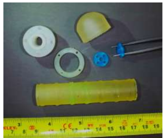
Illustration 3: Samples of each part type for the final version 4 design – a fairlead and a 25mm OD guide ring (translucent white, Formlabs Durable), a friction cap and an 80mm x 19mm OD / 13mm ID core tube (fluorescent yellow, Formlabs Elastic) and two spacer / cable guide 12.3mm x 5mm ellipsoids (blue, Formlabs Tough). All parts printed at 0.1mm resolution.
