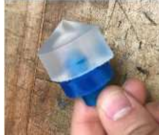
Illustration 5: Fine Grasp Wedge (0.0 mm radius) fingertip printed in Formlabs Elastic material, mounted on a fairlead. Photographed fairlead printed in blue Tough resin for optical contrast in image.
