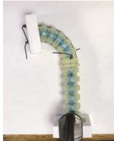
Illustration 6: Testing range of motion with a desktop jig on a two-section tentacle of design version 5.
