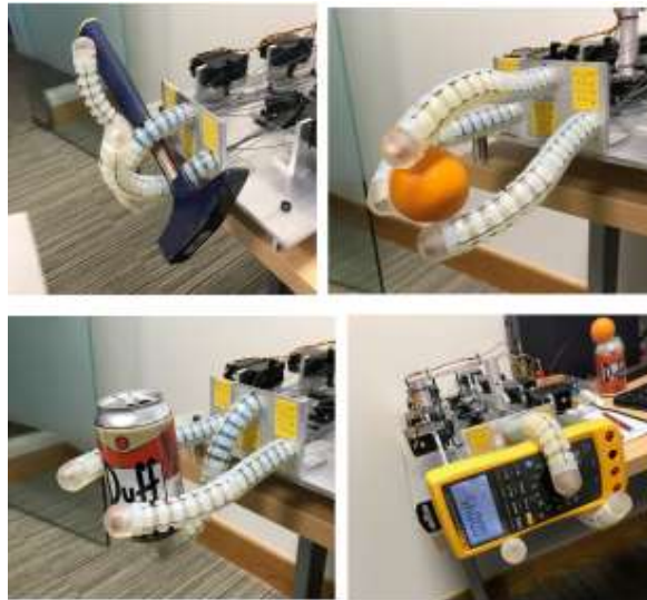
Illustration 8: The Cthulhu-Morphic Gripper grasping common tools and laboratory supplies.
