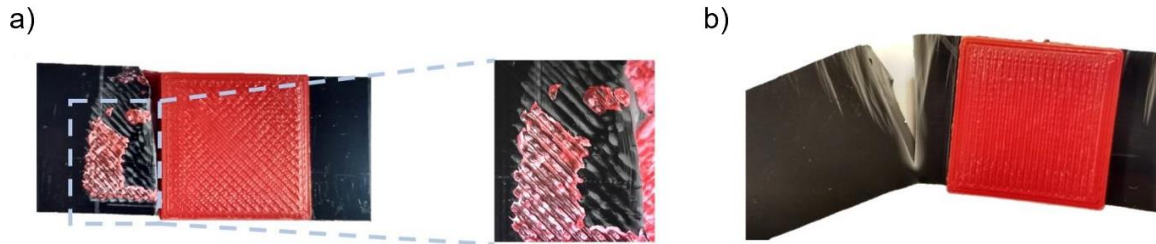
Figure 5: Two modes of failure observed during three-point bending a) Adhesive failure b) Substrate failure
