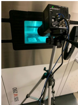
Figure 1. The camera setup outside the EOS M290 process chamber.
