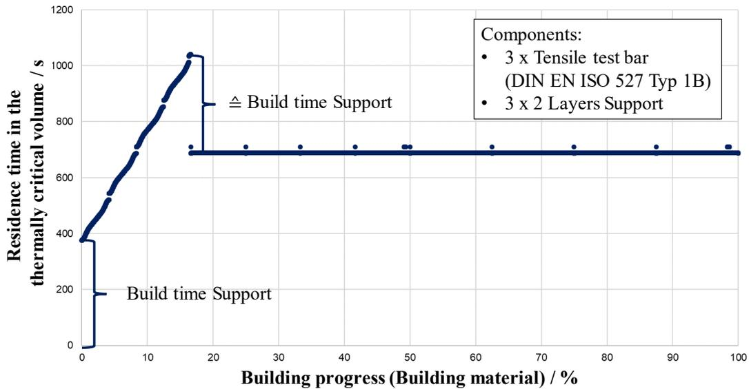
Figure 7: Plot of the data calculated by the software.
