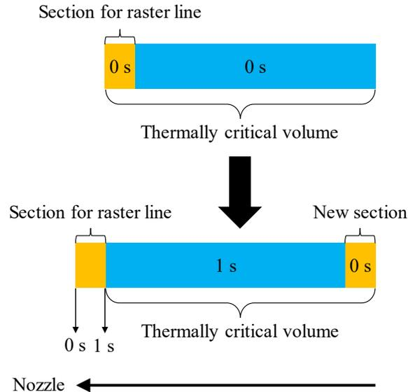
Figure 3: Depiction of the section generation in the thermally critical volume by the software.
