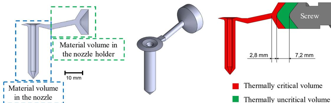
Figure 4: Definition of the thermally critical volume in the Software with an exemplary metering stroke of 10 mm.
