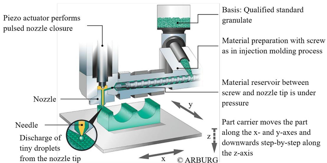
Figure 1: Schematic setup of the Freeformer [1].
