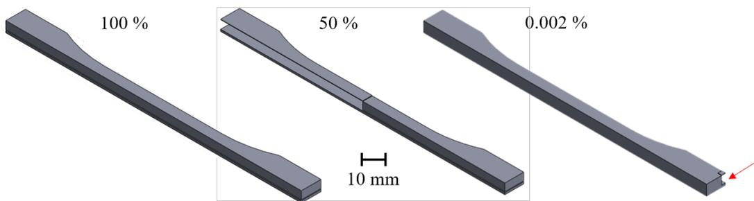
Figure 6: Visualization of the buffer parts as a cross section of the 100 % / 50 % / 0.002 % support material share in the buffer part.
