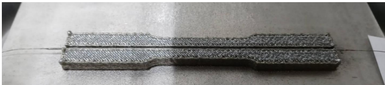
Figure 1: Tensile Specimen and Coated Optical Fiber Before and After Embedment
