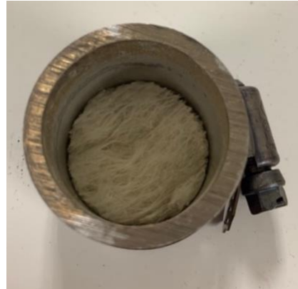
Figure 2: Constraining container and the composite coupon fiber stack
