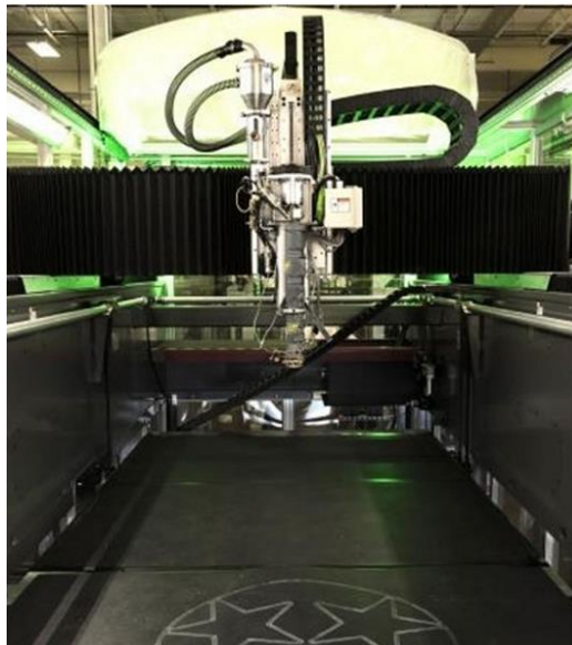
Figure 1: Big Area Additive Manufacturing (BAAM). Example large-scale gantry-based pellet fed polymer system.
