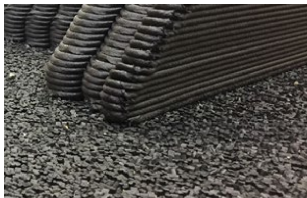
Figure 2: Thermwood's version of a wood board with glued pellets, called "bead board" [6]
