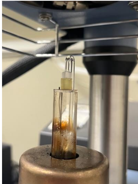
Figure 16: CTE sample puck loaded into TMA Q400
