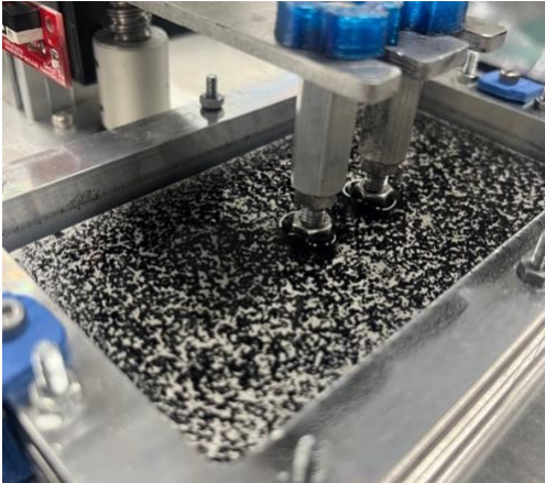
Figure 14: Carbon nanotube conglomeration on print bed
