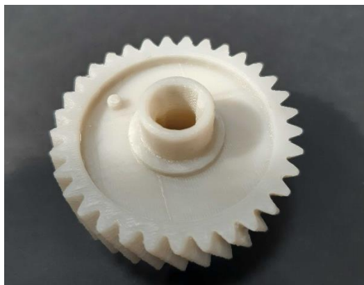
Figure 5: Tracer-based gear wheel. Tracing particles are not visible until excitation with IR light.
