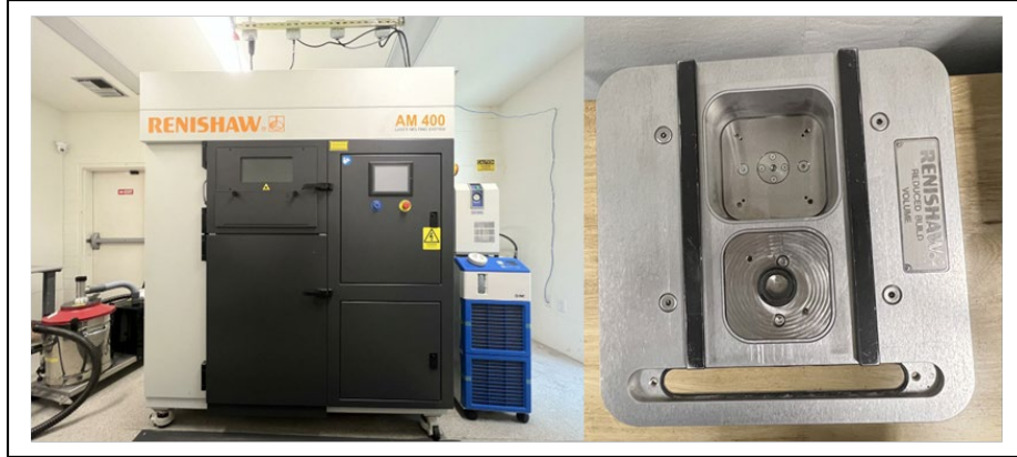
Figure 4. Renishaw AM400 and Reduced Build Volume (RBV) unit
