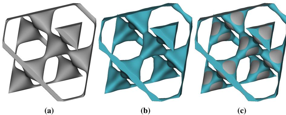
**Figure 7:** Comparison of geometry at 10% volume fraction showing (a) the D-surface, (b) the MC D-surface, and (c) the D-surface and MC D-surfaces overlaid.
