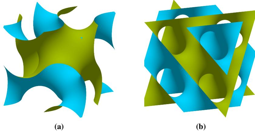
**Figure 1:** Images of the (a) Gyroid and (b) D-surface generated using Surface Evolver with blue and green showing the two sides of the surface.
