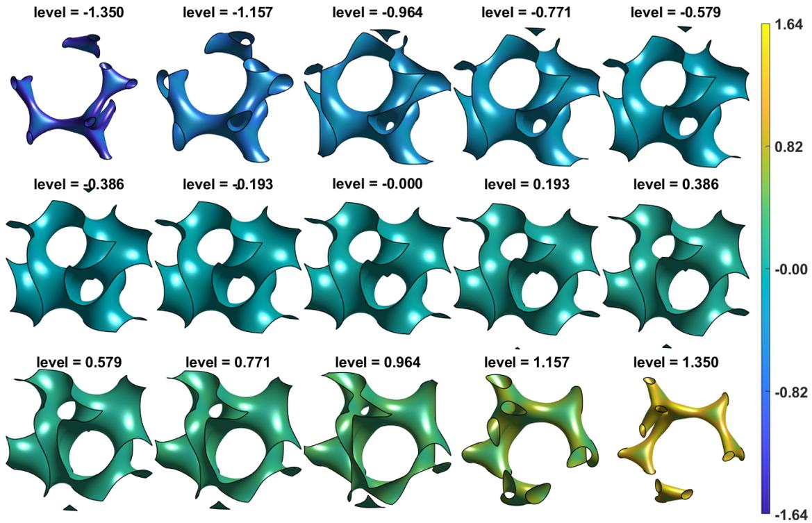
**Figure 2:** Gyroid mean curvature across a range of level sets showing existing nonzero mean curvature, especially when deviating from the zero level set.
