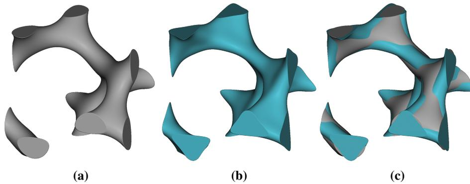
**Figure 6:** Comparison of geometry at 10% volume fraction showing (a) the Gyroid, (b) the MC Gyroid, and (c) the Gyroid and MC Gyroid overlaid.
