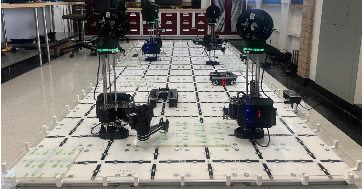
Figure 1: The current iteration of the C3DP system including: i) the SCARA printer and ii) the mobile platform.
