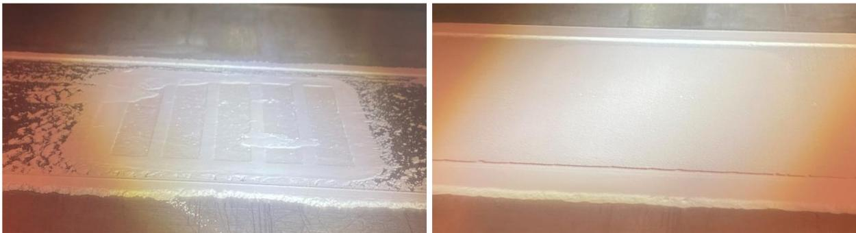
Figure 7: Coated powder of FR dry blends with PMN525 (left) and OP1400 (right)
