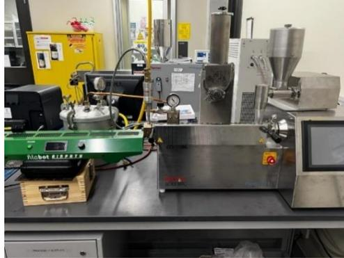
**Figure 4.** Process 11 twin screw extruder
