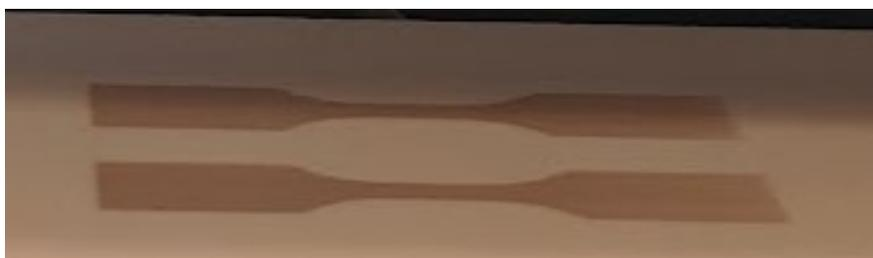
Figure 7: Red color of Activating Fusing Agent visible on powder bed before fusing.
