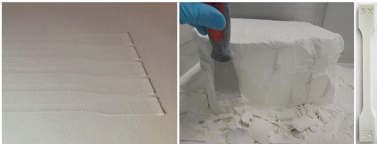
Figure 9: Curling of Specimens at temperatures lower than 188 °C with encapsulated powder (left), pronounced caking of the powder bed with encapsulated powder (middle) and part from encapsulated powder after glass bead blasting (right)
