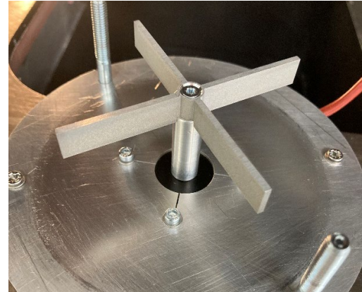
Figure 4 Close-up mixer in-house developed deposition system
