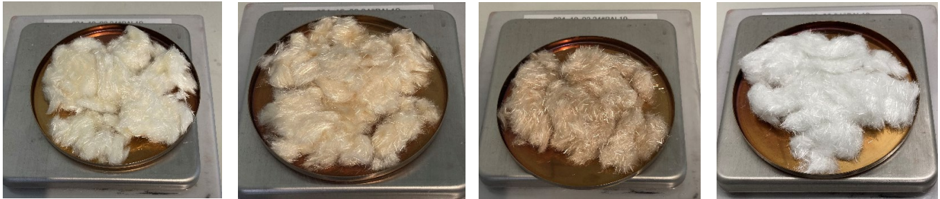
Figure 7 Chopped glass fibres after different heat treatments in air atmosphere (from left to right: 150°C, 250°C, 350°C, 450°C)
