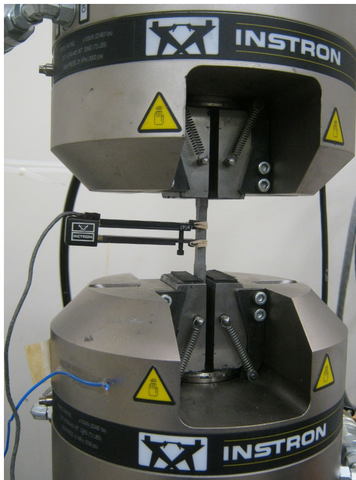
Figure 7: Quasi-static tensile testing specimen and machine setup.
