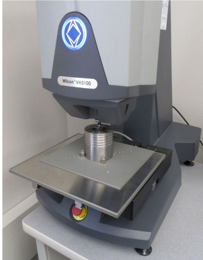
Figure 9: Microhardness mapping setup.
