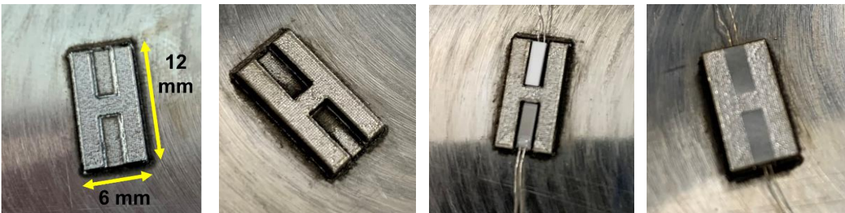
Figure 8: Pt100 RTD embedding from left to right: grooved shape without sensors (first and second images), grooved shape with sensors, and after one layer printed on top of the sensors.
