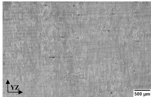
a) Raster melt microstructure in build direction (contrast and sharpness enhanced)
