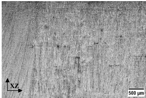
a) Raster melt microstructure in build direction (contrast and sharpness enhanced)
