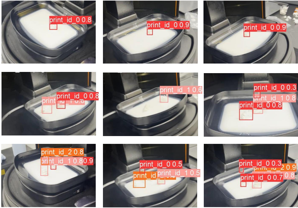
Fig. 5. Qualitative indications of the performance of our object detection model fine-tuned purely on N = 500 synthetically-generated images, for the task of detecting one defect (top), two defects (middle), or three defects (bottom). Numbers adjacent to detected design classes represent approximated confidence scores.
