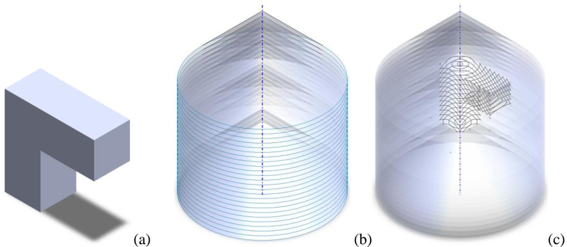
**Figure 3.** Cantilevered “L” part (a), example layer surface stack (b), extracting intersection lines between the part faces and the layer surfaces along with the center axis (c)
