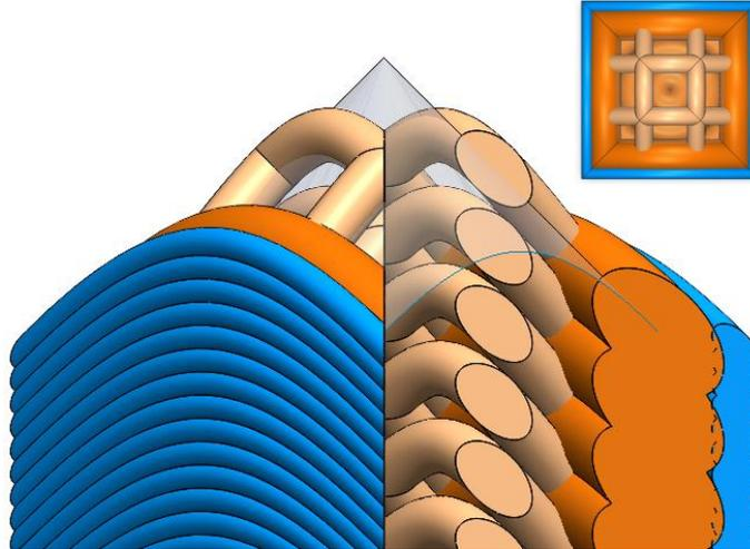
**Figure 1.** Conceptual demonstration of extrusion path types. A virtual cross section of a part mid-print showing an outer shell with fine layers (blue), coarser core perimeters (dark orange), medium thickness low density rectilinear infill (light orange), and the topmost conical core layer (transparent grey). Note that the two core extrusion path types, core perimeter and infill, share a layer surface (the cone) that is not shared by the shell paths. Inset shows top view.
