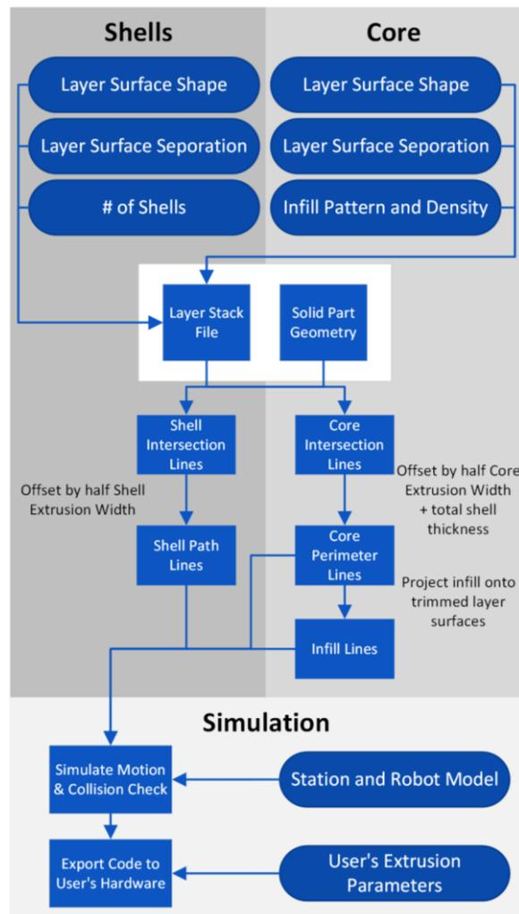
**Figure 2.** The three conceptual sections of this work to generate curved-layer extrusion paths including inputs and flow of dependencies.
