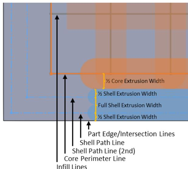
**Figure 4.** Graphical description of line locations and their offsets including Shell Path (2 shells shown), Core Perimeter, and Infill Lines. Shown along the Z axis of the part (“top down”).
