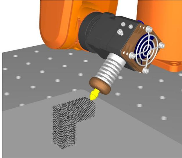
**Figure 5.** RoboDK robot station showing ideal nozzle orientation for that path segment. Core Perimeter Lines shown alone for clarity.
