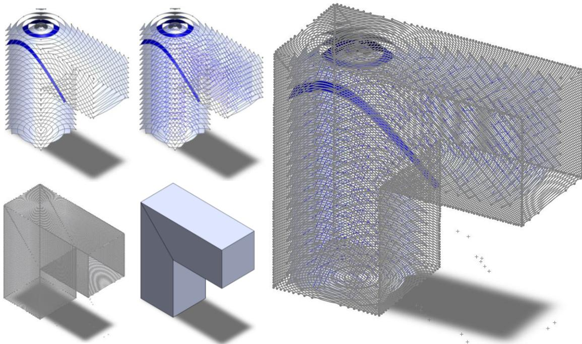
**Figure 6.** Final part using parameters from Section 2.3. Core Perimeter Lines with exemplar blue highlighted conical layer surface (a), Core Perimeter Lines (grey lines) and Infill Lines (blue lines) (b), Shell Path Lines only (c), original solid part (d), all three path types assembled (e)
