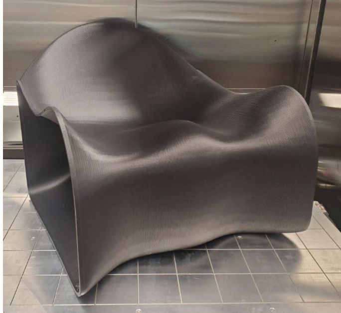
Figure 6: A chair 3D printed using g-code with geometry information.
