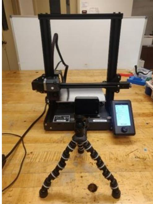
**Figure 11:** Experimental setup to record extruder carriage movement
