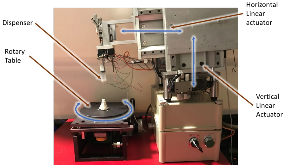
Figure 4 : 3D Printer Schematic
