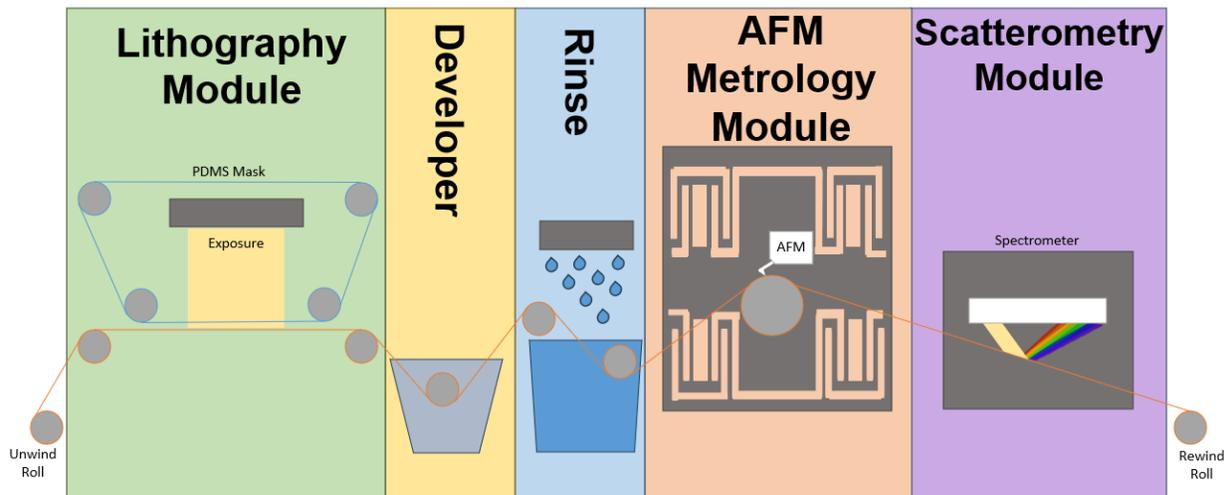
Fig. 9 Diagram of combined manufacturing and metrology system
