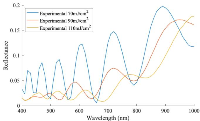
Fig. 8 Reflectance measurements of fabricated samples with 70, 90, and 110 mJ/cm<sup>2</sup> exposure dose versus wavelength.
