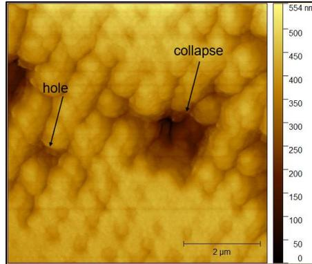
Fig. 7 Static sc-AFM scan of 60 mJ/cm<sup>2</sup> exposed sample
