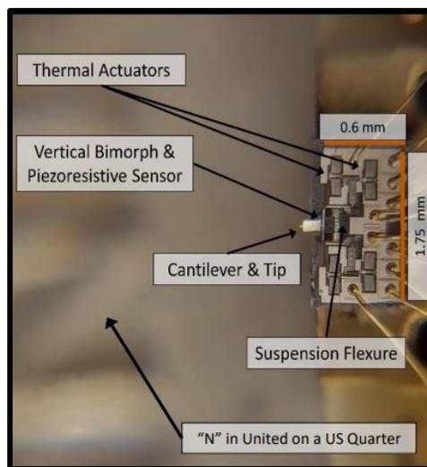
Fig. 6 MEMS sc-AFM [8]
