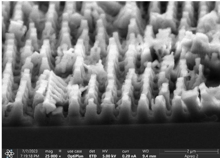
Fig. 4 Final image of 3D holographic lithography pattern
