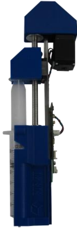
Figure 3: Hyrel Syringe Deposition Device [6]
