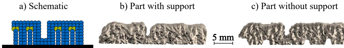
Figure 13: TUM logo with salt release layer support structure. Schematic (a), printed part with support structure (b), and printed part after support structure removal (c).
