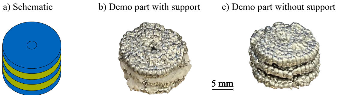
Figure 10: Demo part, fabricated according to the AlSi12 on AlSi12 sequence. Schematic (a), printed part with support structure (b), and printed part after support structure removal (c).
