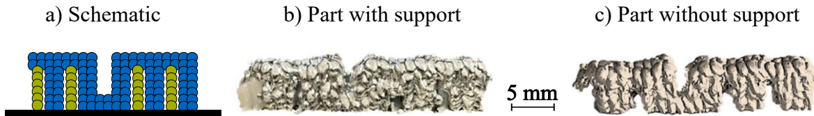
Figure 12: TUM logo with salt pillar support structure. Schematic (a), printed part with support structure (b), and printed part after support structure removal (c).
