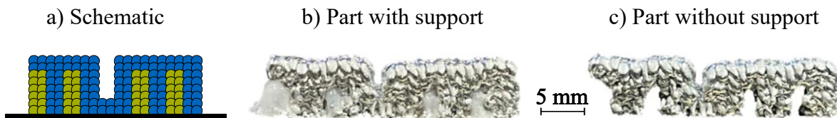
Figure 11: TUM logo with monolithic salt support structure. Schematic (a), printed part with support structure (b), and printed part after support structure removal (c).
