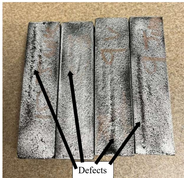
*Figure 8: Defects shown in parts cast from gyroid-filled patterns*
