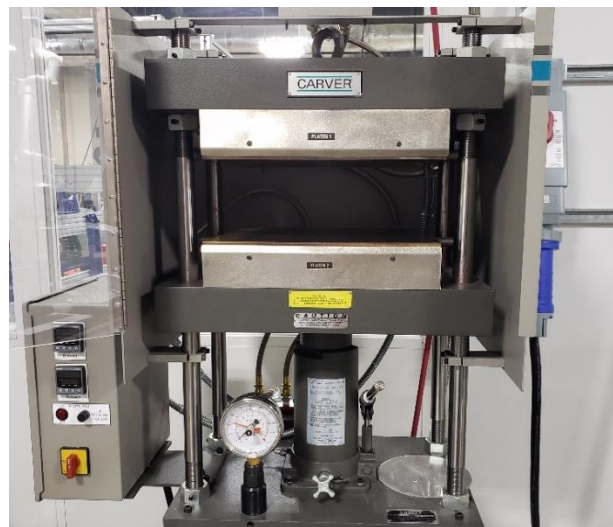
Figure 2. Compression molding of 3D printed preforms was completed using heated hydraulic press.
