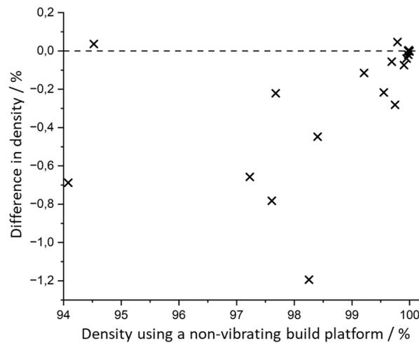
Figure 2: Difference in relative density (density using a vibrating build platform – density using a non-vibrating build platform) plotted over relative density of samples manufactured using a non-vibrating build platform.
