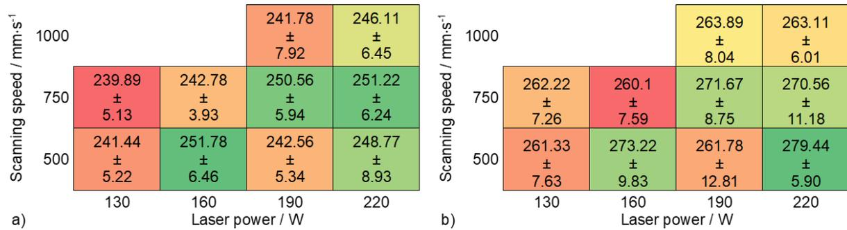
Figure 3: Hardness with standard deviation in HV 1 of samples manufactured a) using a non-vibrating build platform and b) using a vibrating build platform.
