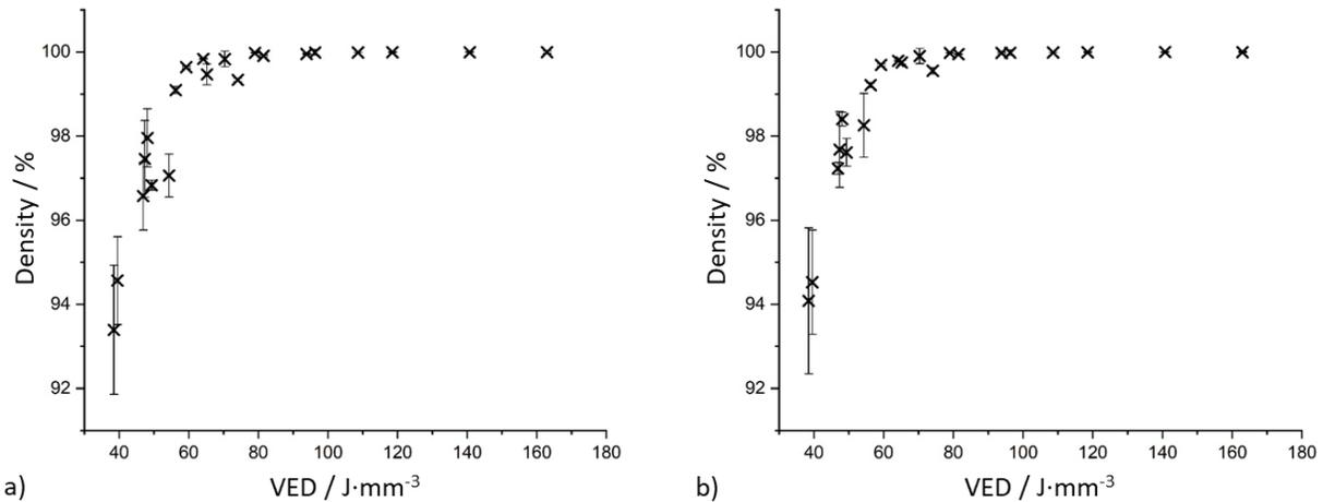
Figure 1: Relative density with standard deviation plotted over volumetric energy density a) without using a vibrating build platform, b) using a vibrating build platform.
