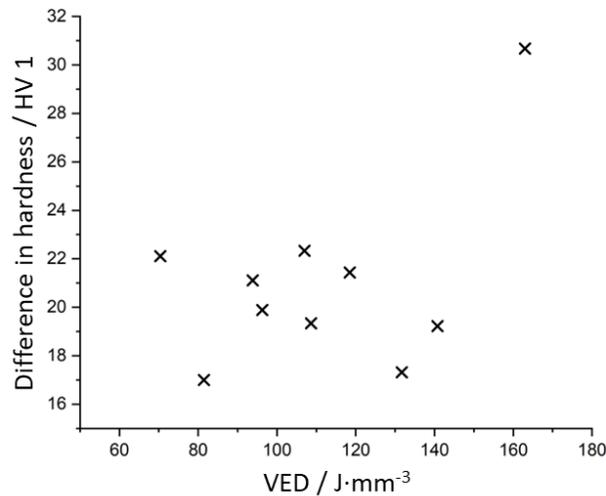
Figure 4: Difference in hardness (hardness using a vibrating build platform – hardness using a non-vibrating build platform) plotted over volumetric energy density.
