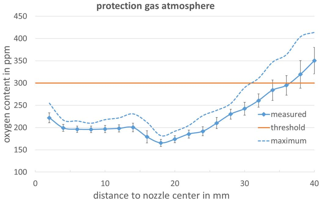
Figure 3: Oxygen content in respect to the distance to the center of the nozzle
