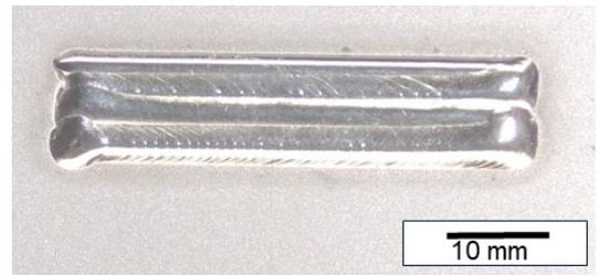
Figure 4: Ti-6Al-4V weld
