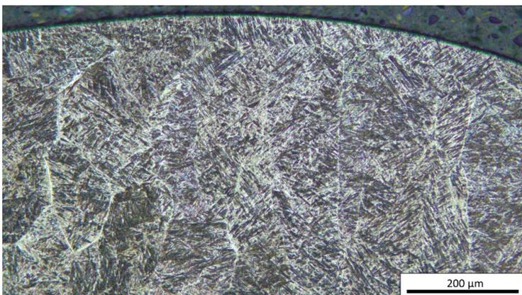
Figure 5: Microsection of the welded Ti-6Al-4V sample
