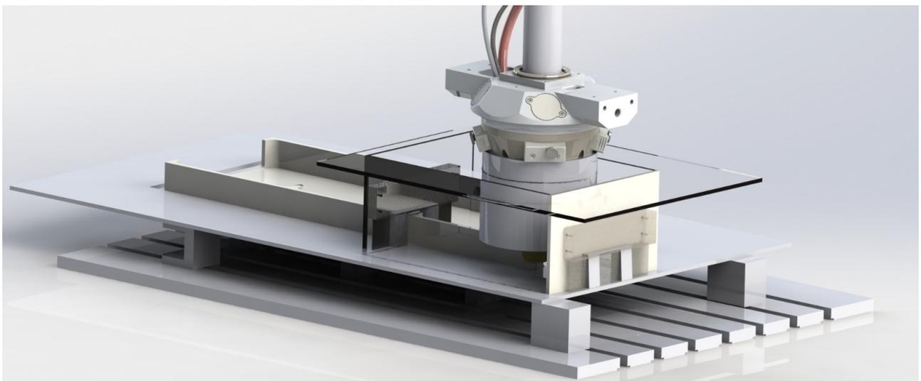
*Figure 1: Rendering of the protection-gas chamber on a planned work piece with adaptive seals and partly immersed laser-head.*
