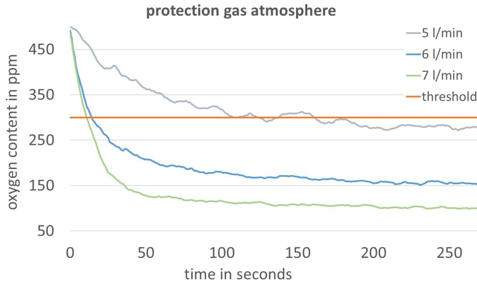
Figure 2: Oxygen decay in protection gas atmosphere for different argon flow rates
