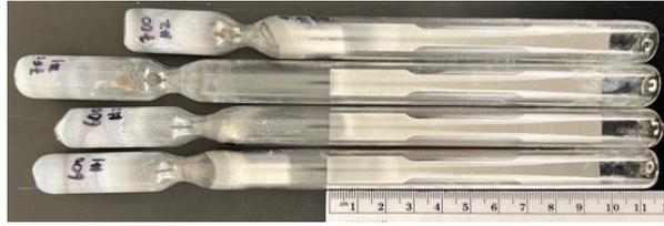
Figure 1. An evacuated quartz tube with LDED 316Y tensile specimen and Zr (as oxygen absorber) subjected to thermal stability test
