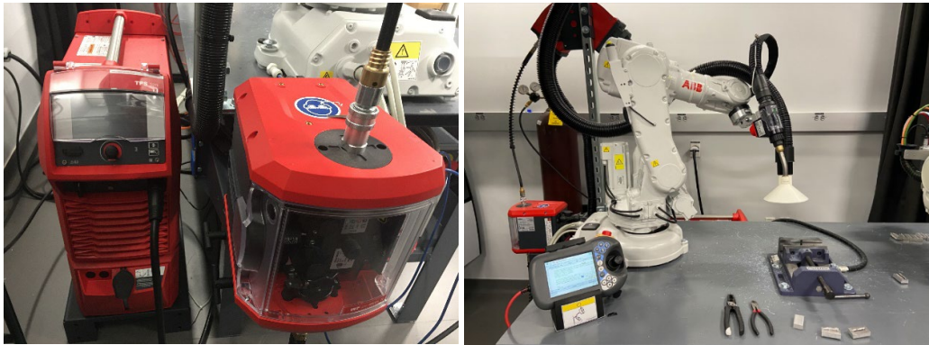
Fig 4 Fronius welding system (left) and ABB robotic welding arm (right) used in the experiment
