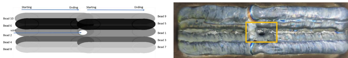
Figure 4: Schematic representation of top layer of a multi-layer multi-beads printing (left) and Actual printing (right).
