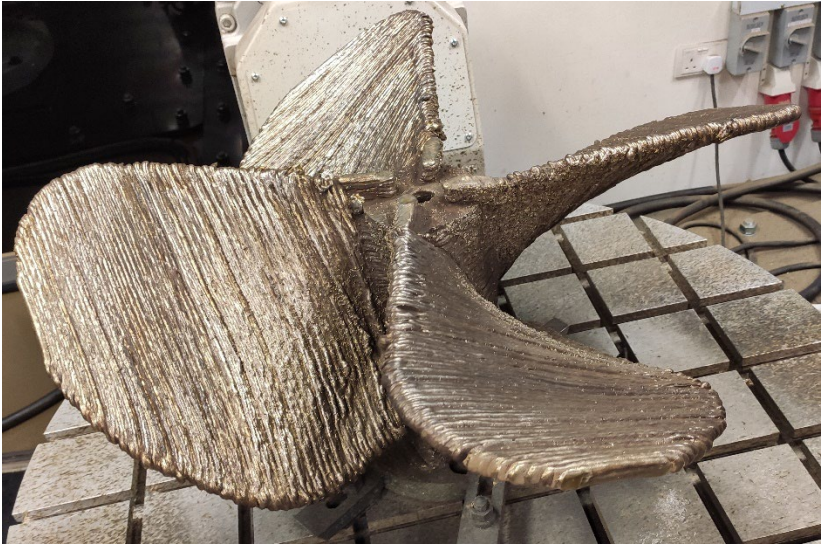
Fig. 7: Propeller printed using multi directional printing approach
