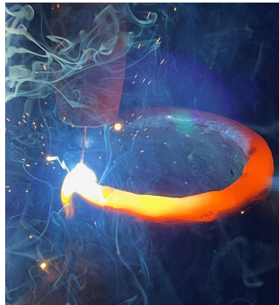
Figure 3. WAAM process executed on a Fanuc six-axis robot.
