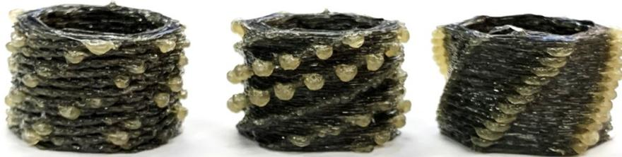
Figure 5: Printed specimen (15°, 5°, 1.25° pitch angle from right to left)
