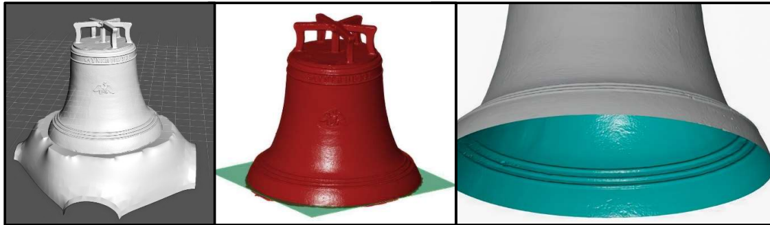
Figure 16: Bell mesh before cutting (left), bell with cutting plane in “GOM Inspect“, bell after cutting base [14]
