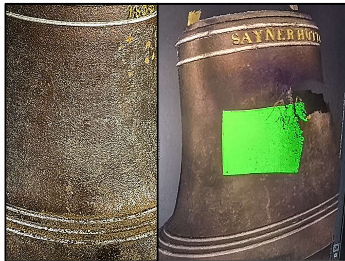
Figure 8: Typical cast-iron surface of the bell (left), optical feedback when scanning the cast iron surface of the bell (right), [14]
