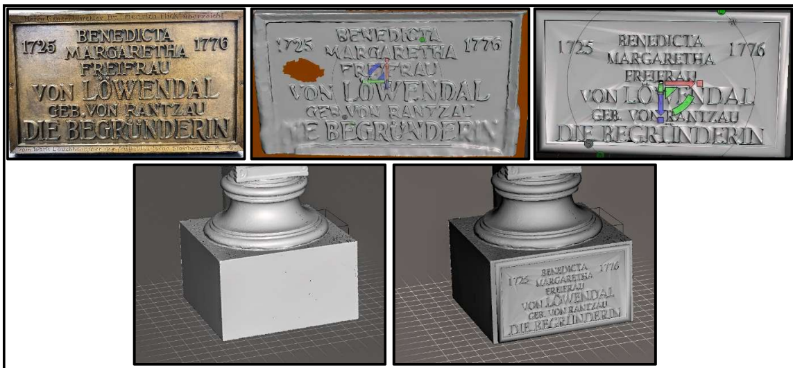
Figure 19: Original inscription (top left), scanned inscription (top middle [14]), modelled inscription (top right [14]), base with deleted inscription (bottom left [14]), base with modelled inscription added (bottom right [14])
