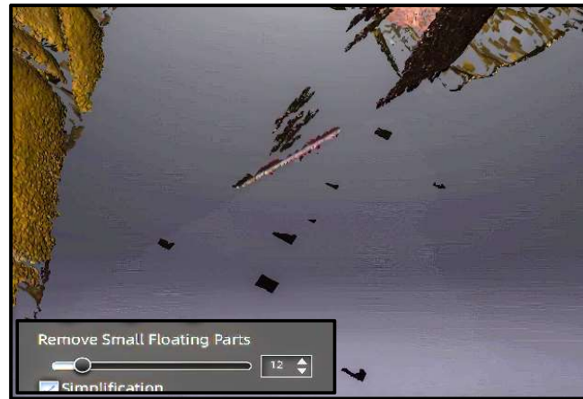
Figure 12: Floating parts in the point cloud of the eagle, “ExStar“ meshing option
