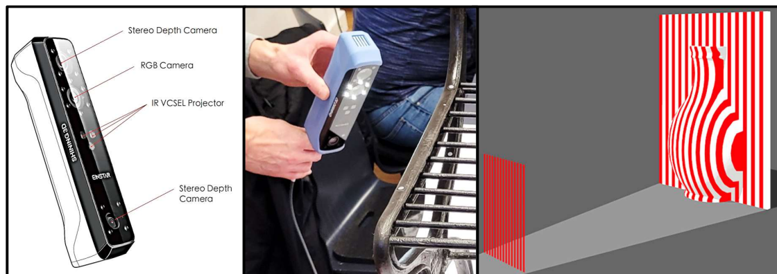
Figure 6: "Shining EinStar 3D" Scanner (left [5], middle), distorted light pattern (right [2])
