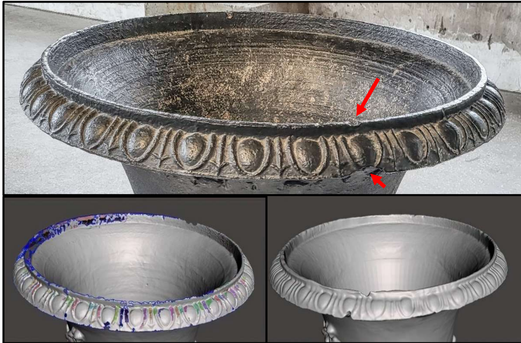
Figure 14: Manual modification of vase details representing the original (faulty) structure: (a) original vase, (b) meshed surface in “MeshMixer“, (c) manually closed holes [12]
