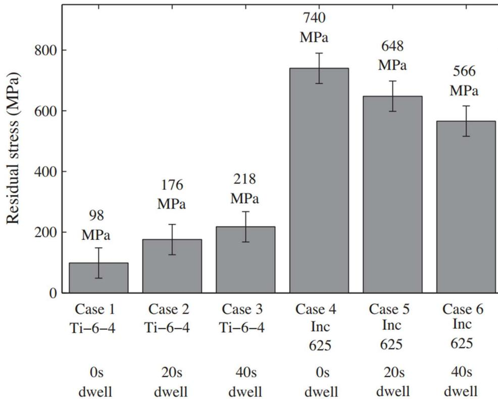
Figure 1. Variation of residual stress evolution with inter-layer dwell time in DED of Titanium and Nickel alloys; with permission from publisher [8]
