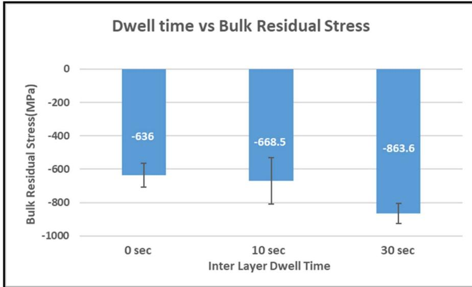
Figure 8. Variation of bulk residual stresses with inter-layer dwell time
