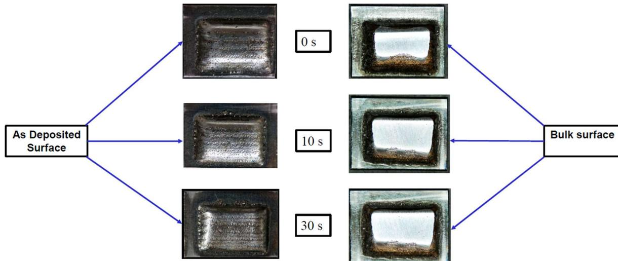
Figure 6. High Strength Steel Alloy specimens deposited by laser DED
