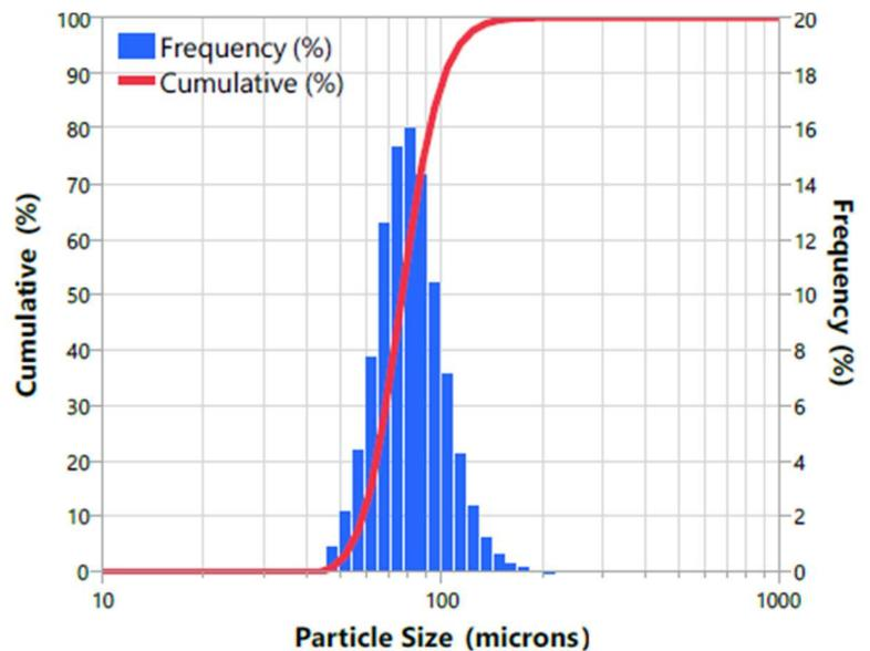
Figure 2. a) SEM image of High Strength Steel Alloy powder. b) Particle size distribution of Alloy powder
