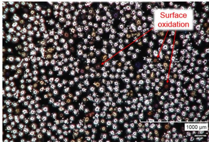
Figure 3. Optical microscope image of High Strength Steel Alloy powder
