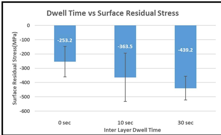
Figure 7. Variation of surface residual stresses with inter-layer dwell time
