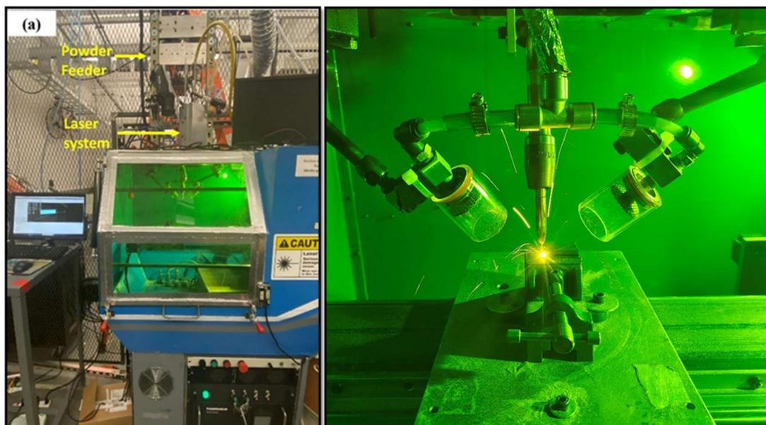
Figure 5. Laser DED system used for deposition.
